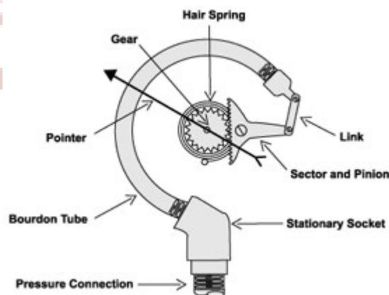
Oil-filled bourdon tube gauges use a sealed tube in an oil-filled housing, in this case the pressure transmitted by the oil to the tube causes it to tighten and move the depth gauge needle. These are better as they are not prone to clogging.
